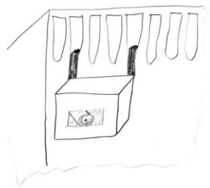
Figure 1. Camera mount with hooks to attach to the chamber wall.
